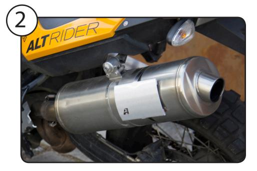
Fit up to your bike and tighten the hose clamp with a 8mm socket. You will need to test fit your luggage to make sure that the luggage is only touching the heat shield and not some part of the hot exhaust pipe. Try to position the clamp so that the fastener is hidden behind the exhaust when fully tightened. Adjust as needed.
