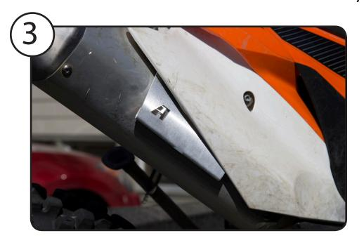
If you are installing on a dirt bike or between the fairing and the exhaust, it is much easier to dry fit the shield before adding the hose clamp.
