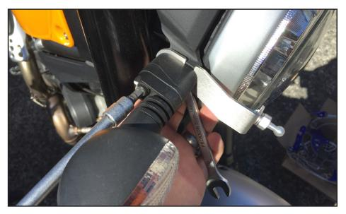
Place the arm with the slot facing UP as shown in the photo. Using the OEM hardware, insert the M6 and have the nylock nut ready to receive it. Tighten this hardware down, leaving one or one and a half turns so you can reposition the arm later in the process. Repeat this process for the left arm.
