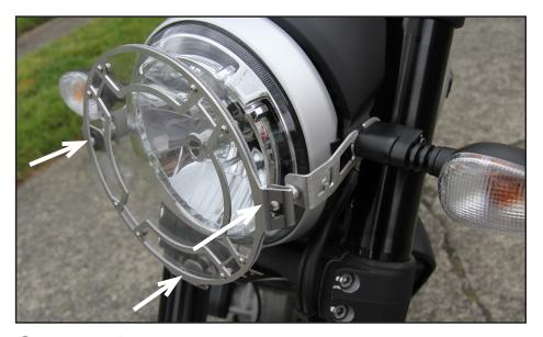
Finally, carefully press the rubber grommets over the ball studs. You can do this one at a time by applying pressure to the areas indicated. Apply some form of lubricant to the rubber grommets (even some water will work) and then use the heel of your hand to press each ball stud into the sockets.
