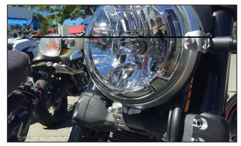
Now that all (3) bracket arms are in place, check the position of the left and right ball stud ends. Use a straight edge if you like to align the left and right arms so that the ball studs are roughly aligned with the center point of the headlamp. Using the 10mm wrench and 5mm allen tool, complete the tightening of the OEM M6s to secure the arms.
