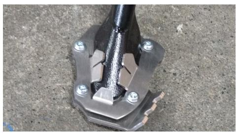
Tighten the rear 12mm screws so that the top plate squeezes the side stand tight. The stack of washers prevents over tightening.
