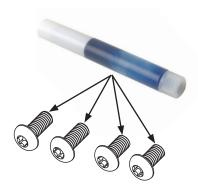
Apply thread locker to the tips of all four screws. **TIP:** To make installation easier, have a friend balance on your bike with the side stand off the ground. Or put your bike in gear and lean it against a sturdy wall.
