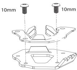
② Loosely thread in the two M5 x 10mm long screws through top plate and into bottom plate in locations shown. Only screw in a few threads, screw should not extend below bottom plate.
