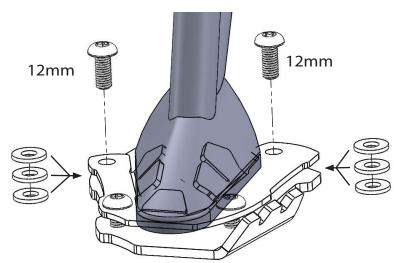
3 Slide onto side stand. Place washers between upper and lower plate as shown, three on each side. Hold plates aligned and thread in M5 x 12mm long screws.
