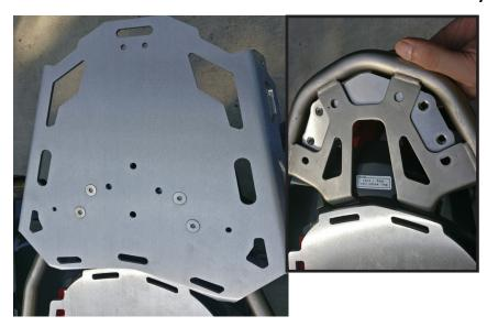
Place rack on top of OEM platform. Mounting holes should line up with bracket as shown.
