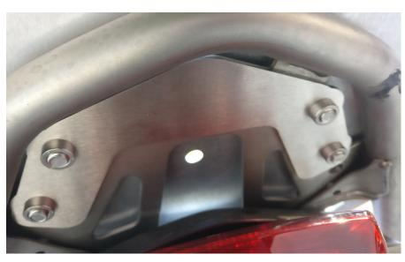
2 Insert (4) M8 screws and tighten each bolt 15 Nm into bracket. TIP: Before tightening all the way ensure Luggage Rack is properly aligned.
