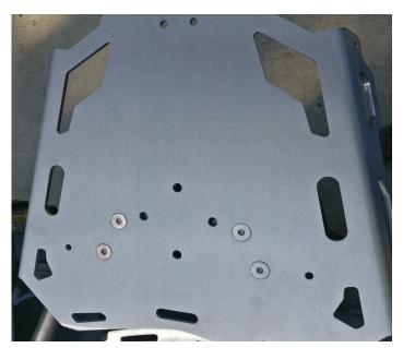
3 After 5 hours of riding, or 100 miles, check all the fasteners on the assembly to ensure they are tightened to spec.
