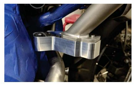
Next, install each billet block into their respective upper crash bar ange using the (2) M6x 16 socket cap screws, (2) M6 washers, and thread locker. Tighten to 8Nm
