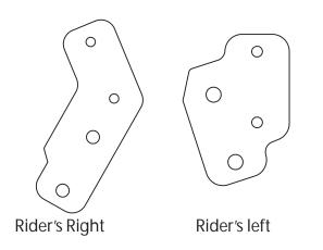
Once AltRider upper crash bars are installed, separate the kit contents to each side. Note the di erence in shape for each side of the billet peices.
