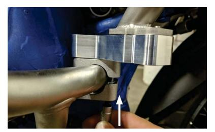
Rest the top half of the clamp onto the OEM crash bar. Apply thread locker thread to the M6x50 (riders right) and M6x 45 (riders left) and install M6 washers. Carefully hand thread the fasteners through the bottom clamp half, passing through the top half, and into the threaded billet block as shown.
