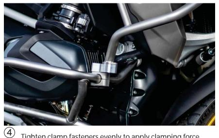
7 Tighten clamp fasteners evenly to apply clamping force on OEM crash bar. Tighten fasteners to 8Nm.
