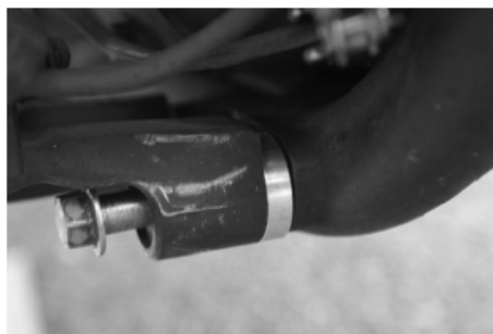
Fig. 2 – Floorboard Mount Spacer Installed
