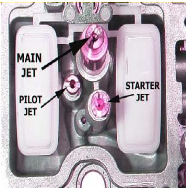
9. Thoroughly clean the inside of the float bowl prior to reinstalling it.
