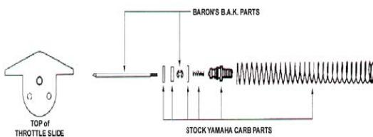
5. Reinstall the vacuum slide along with the diaphragm spring.
