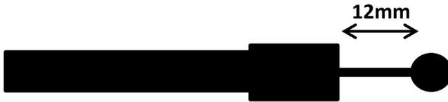
**When attaching the barrel cable clamp to the remote wire, make sure you pull on the end of the shift cable, so that there is no play in the remote lever. Then clamp the barrel at 12mm free wire length from the endcap!**
