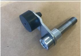
2. Use 8mm allen and remove the front bolt of the rear cradle mount on the left side of the motorcycle.
