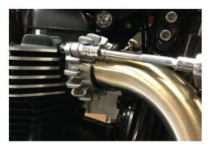
8. Tighten clamps on catalytic converter to 8 Nm. (70 in-lbs) NOTE INCH-POUNDS
