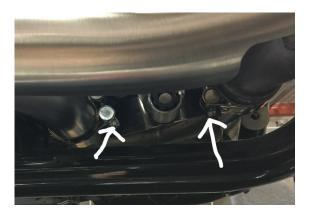
9. Install heat shield to tailpipe.
