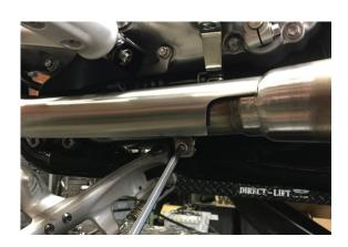
10. Reinstall Rear Brake Clevis onto shaft. There is dot on the shaft and hole in the clevis to ensure proper alignment.
