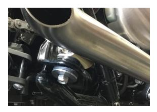
Use 12mm socket to tighten head pipe flange nuts and torque to 19 Nm (14.0 ft-lb)
