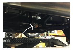
3. Place kickstand stopper bracket into position and secure with supplied hardware.
