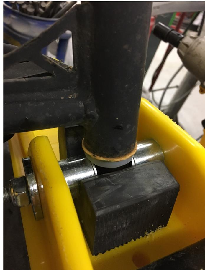
6. Install ski onto sled by centering the hole in the dampener with the lower part of the spindle. This will allow you to now install the bolt, washers, and nut. (see picture).
