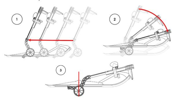
6. When the handle and saddle are in place, and the Sled Wheels assembly is installed onto the ski, the latch should swing open and close around the ski loop. Slide the latch up until it just touches the ski loop and tighten the screw. Do not over-tighten.
