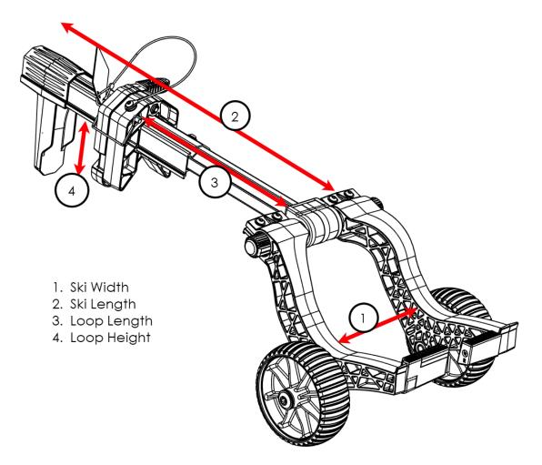
1. If not done previously, adjust the width of each Sled Wheel assembly to be approximately ½" wider than the ski. Include space to avoid the spindle screw if it sticks out past the ski. Tighten, but do not over tighten the arm clamp screws.
