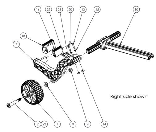
bolt (or cut the excess bolt off). The arm angle can be adjusted  $15^{\circ}$  to accommodate tall or short ski loops. Most sleds work best at  $15^{\circ}$ . Use two  $\frac{1}{4}$ -20 x 1.0" (13), two  $\frac{1}{4}$ " washers (15), and two  $\frac{1}{4}$  square nuts (14) to secure the arms in place using the supplied  $\frac{5}{32}$ " hex wrench (8). Do not overtighten. Make sure both arms are installed at the same angle.
