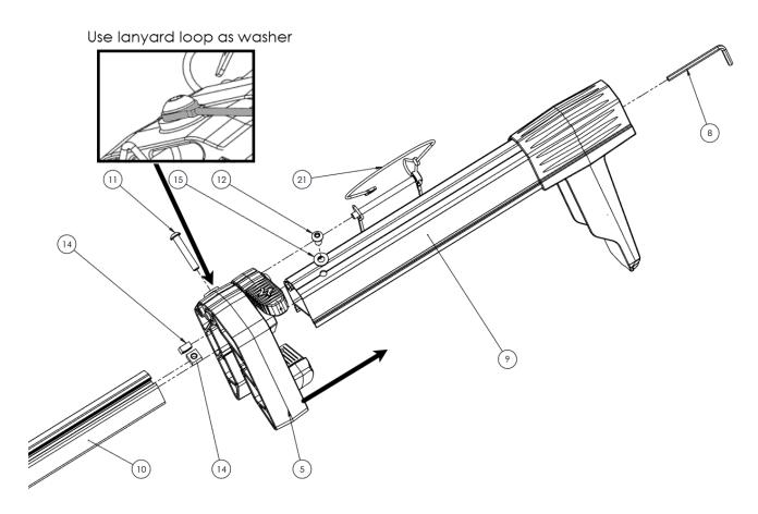
7. Place a ¼" square nut in the T-slot of the T-Handle and then slide a Telescoping handle onto the T-handle, lining up the nut with the hole in the Telescoping Handle. Secure the handle about 6" extended with a ¼-20 x 0.5" screw (12) and ¼" washer (15). The extension will be adjusted to the ski later.
