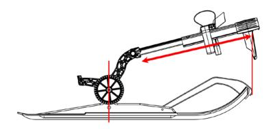
3. Adjust the saddle/latch assembly so that the latch will close at the peak of the ski loop. Tighten the saddle screw.
