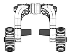
3a. For skis that are flat or have even runners, assemble the short finger covers (16 and 17 - be sure to use the left cover on the left arm, and right on right). Tap the rubber on a hard surface to ensure it is fully seated. Secure with a self-tapping screw (20).
