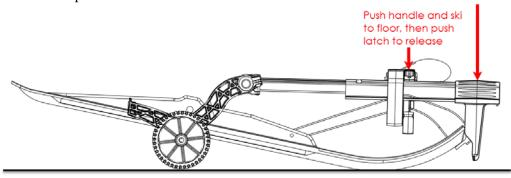
2. Slowly move the handle up. Remove Sled Wheels from the ski, lifting the ski loop if necessary. Close latch and replace safety pin. Store fully assembled, ready for your next ride!
