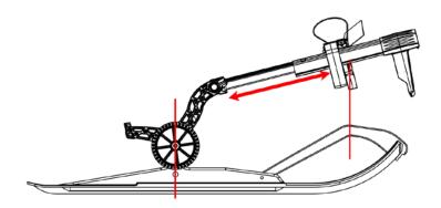
4. Loosen the latch adjustment screw three turns so that the lower portion of the latch is moveable.
