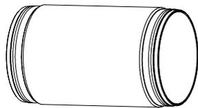
Apply thin layer of waterproof grease to ends that go inside BB cups
