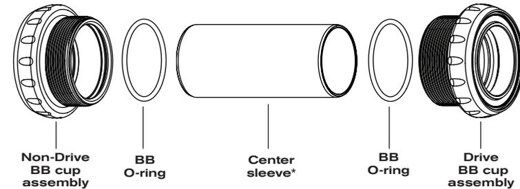
\*Chris King ThreadFit™ 24 bottom brackets ship with a center sleeve for a 68/73mm bottom bracket shell. For all other bottom bracket shell sizes, the correct center sleeve will be supplied with the appropriate conversion kit.
