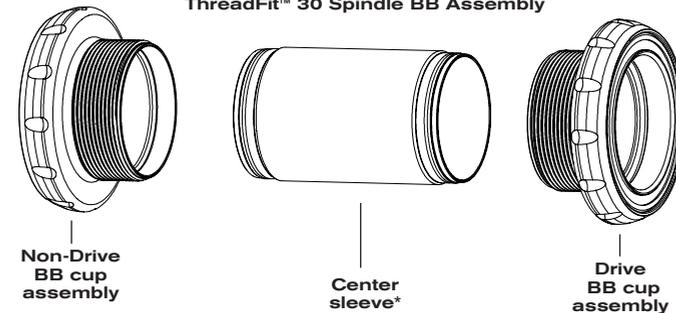
\*Chris King ThreadFit™ 30 bottom brackets ship with a center sleeve for a 68/73mm bottom bracket shell. For all other bottom bracket shell sizes, the correct center sleeve will be supplied with the appropriate conversion kit.
