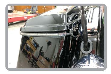
5. Remove adhesive backing from tape and install Bag Blade onto saddlebag, one side at a time. Press and hold firmly for 60 seconds. Adhesive fully cures within 24 hours.
