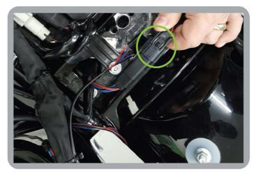
8. Plug the Bag Blade wires into the controller harness. The right Bag Blade should plug into the side of the controller with a brown wire and the left Bag Blade should plug into the side of the controller with a violet wire. Turn on accessory power to verify that the lights are functioning correctly.
