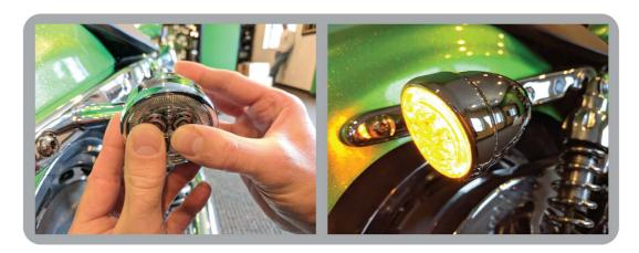
6. Turn on ignition and check for proper turn signal function.
