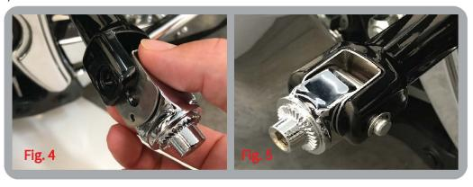
6. Slide the OEM pivot pin through the mount and adapter. Reinstall the clip. (Fig. 5) G0060015, REV. -
