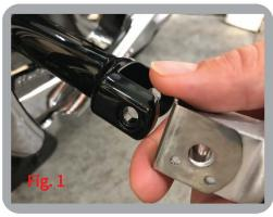
3. Slide the steel detent plate off the footrest to release the ball and spring. Be careful - the ball is spring loaded and can fly out.
