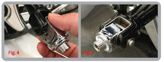
6. Slide the OEM pivot pin through the mount and adapter. Reinstall the clip. (Fig. 5)
