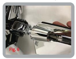
8. Using a 1/4 Hex wrench to hold the screw in place, align the screw threads with the female threads in the adapter, then tighten.
