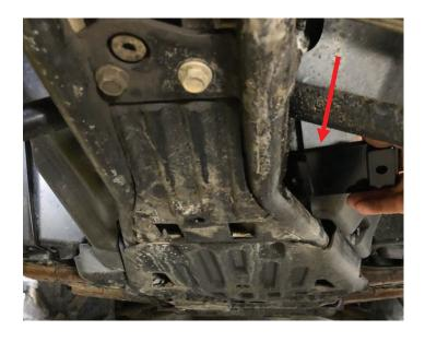
3. Make sure that the rectangular shape goes through the opening of the skid plate.
