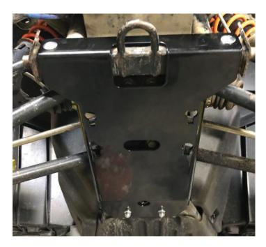
8. Put the 4 carriage bolts (4) through the holes of the V plate (7) with the nuts (4). Tighten by hands.
