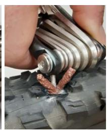
3. Push the fork tool and tire plug into the puncture so it is about halfway inserted.4. Hold the tire the fork tool.
