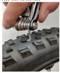
1. Insert the fork tool into the tire and rotate to prepare the hole for sealing.
