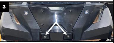
5. Using the provided License Plate Mounting Screws, install the license plate.
