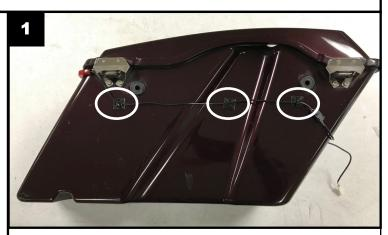
BAGZ<sup>™</sup> come with plug and play weatherproof quick disconnect to make future removal of saddlebags quick and easy (see pictures below).
