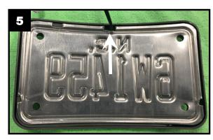
7. Route the wires of the license plate frame through the hole in the mounting bracket as shown in Picture 6. Using the 4 provided license plate frame screws, install the license plate and frame onto the mounting bracket.
