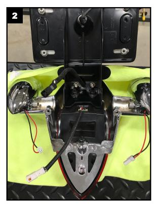
4. Remove the 2 bolts and spacers securing the stock license plate mount to the taillight housing. Retain the bolts and spacers as they will be used for reassembly. Refer to Picture 3.
