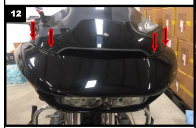
Once the windshield fasteners and windshield are removed, you will need to remove the vent. The vent is secured to the fairing by clips. Position yourself in the front of the motorcycle and lift straight up on the vent to release. Refer to Photo 13.
