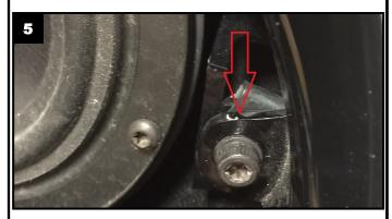
Locate and remove the lower T-25 screw on each side of the inner fairing. Refer to Photo #6
