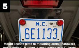
not included), if using in conjunction with Custom Dynamics® Illuminated plate frames or Tag Bolts, mounting hardware is included with these products.
