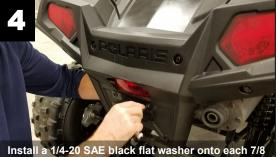
black cap screw, then insert into the bracket and facia. Next, install the lock nuts, tighten with a 4 mm Hex key and an 11 mm wrench or socket.
