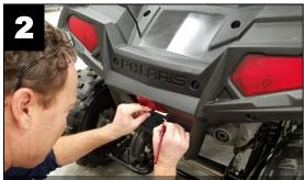
Fit test bracket, draw guide marks for the drill holes in the desired area. Pay attention to level and center for the best fitment.
