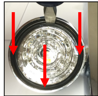
Gently pry around the perimeter
