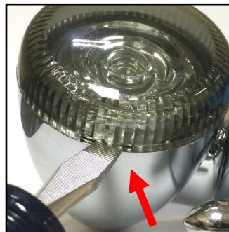
Remove Lens at the slot
