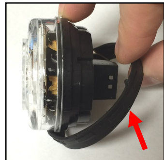
Remove the black gasket from around the stock LED assembly
