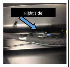
10. Disconnect 2 pin factory wire harness to the Tour Pak® lights.
