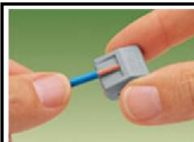
Strip wire 9-10 mm. Use wire gauge on bottom to verify.
