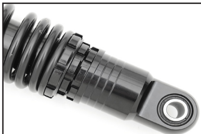
Figure 2. Lower shock with shock shortened to minimum length.
