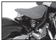
**WARNING!:** Inspect all studs for correct length, considering compression and distance of travel. If there appears to be any interference of travel, remove springs, trim studs and reinstall.
