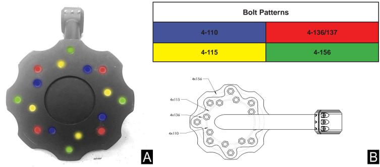
**Step 2:** After identifying your bolt pattern, place a hex bolt(P2) in each hole from the rear. You may verify the bolt pattern by placing your wheel flat on the ground and putting on the spare tire carrier with bolts. Make sure each bolt is aligned with the wheel bolt holes. (Figure C)
