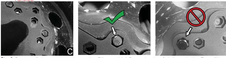
**Step 3:** Once you verify the correct pattern, place a push nut(P3) onto each bolt. Press each push nut firmly down to the plate. These will be pressed down also when putting on your wheel. (Figure D)
