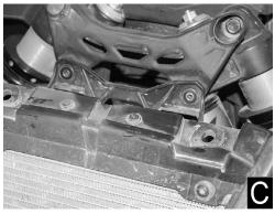
**Step 5:** Place light bracket between the radiator housing and the suspension bracket (Figure D). Align the bottom slot of the light bracket to the holes on the vehicle and then install factory hardware removed in Step 4. Leave hardware loose.
