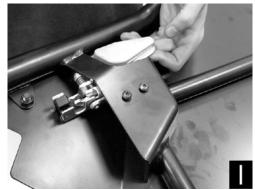
**Step 12:** Remove factory striker pin (Figure J). Retain 2 factory bolts for reuse. The factory striker pin will be replaced.
