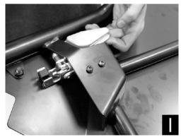
Step 12: Remove front factory striker pin (Figure J). Retain 2 factory bolts for reuse. The factory striker pin will be replaced.
