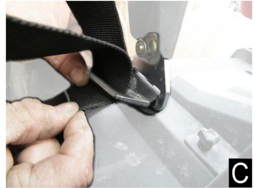
**Step 7:** Finally, route the end of the belt back through the front of the top slot on the buckle to prevent slipping. (Figure D) Pull webbing completely through until tight. (Figure E)
