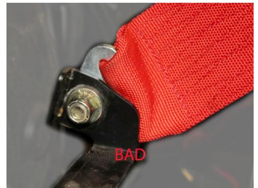
**Step 4:** With seat still removed, install the shoulder portion of the harness to a harness bar, bracket or harness anchor system, by placing the end of the shoulder harness under the bracket or tube attachment point and looping back over. (Figure A, hanging bracket shown)
