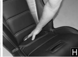
Step 10: Test seat slider by hand, ensuring the seat pan slides correctly and the pin fully engages gate with tension still on the spring.
