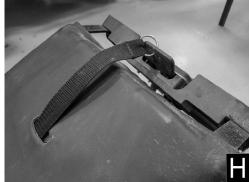
**Step 10:** For 2 seat models and the rear seats on 4 seat models, attach the ring connected to nylon strap on the back of the DragonFire Seat to the seat base release handle (Figure H). Some seat handles may require drilling a larger hole to accept ring.
