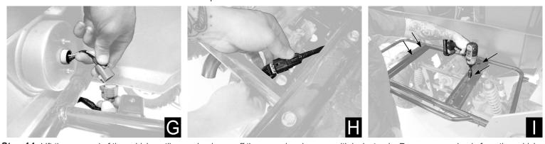
Step 14: Lift the rear end of the vehicle until rear wheels are off the ground and secure with jack stands. Remove rear wheels from the vehicle.
