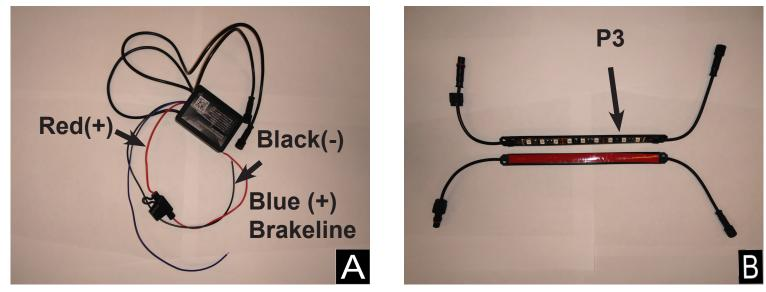
**Step 4:** Install the bluetooth box and route the wiring to the locations for mounting your lights. Make sure to hook up the red wire (+) and the black wire (-) ground to the correct power bar connection. (**Figure A**) The blue wire is to be connected to the (+) side of the brake line wires. When braking happens all the lights will change to red.
