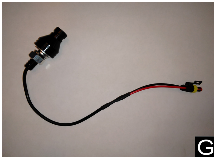
Supplied connector wired to whip light quick release.
