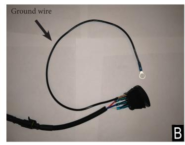
**Step 4:** Install the rocker switch provided and route the wiring to the locations for mounting your lights. Make sure the rocker switch is grounded properly on the frame or negative side of the power bar. (**Figure B**).
