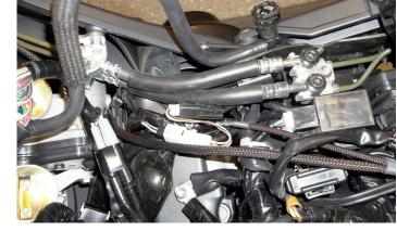
9 Unplug the stock Throttle Position Sensor (TPS) connector.
