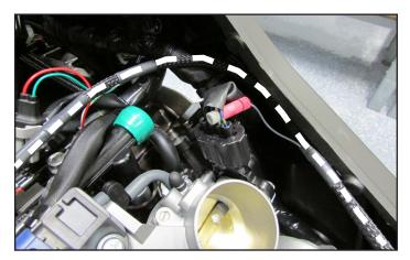
12 Unplug the stock wiring harness from all three of the bike's Fuel Injectors.
