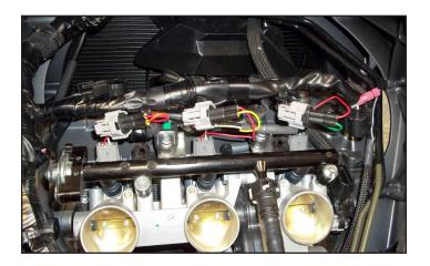
13 Plug the PCV wiring harness in-line of each Fuel Injector and the stock wiring harness.
