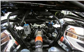
10 Plug the PCV in-line of stock wiring harness and injectors.
