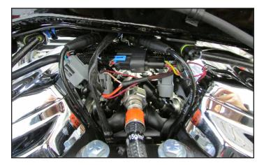
11 Unplug the stock wiring harness from the Throttle Position Sensor.
