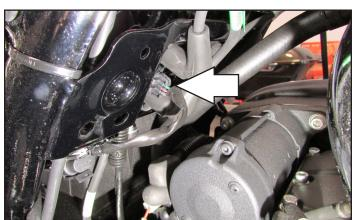
14 Connect the PCV in-line of the stock wiring harness and ignition coil.
