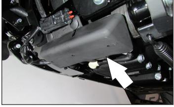
17 Unplug the stock Crank Position Sensor.
