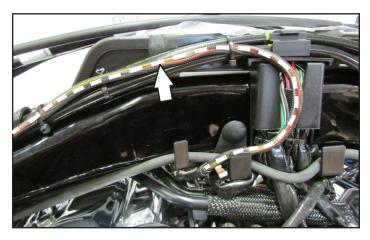
9 Unplug the stock wiring harness from each injector.
