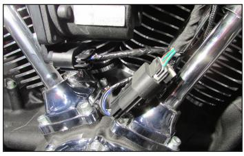
13 Unplug the stock wiring harness from the ignition coil.
