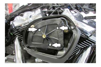
5 Remove the air cleaner and the airbox backing plate.
