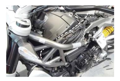
At the air box, route the PC6 wiring harness along the stock wiring harness on the left side. Route harness between the air box and the frame at the front of the bike, and bring the connectors out on the left side of the bike behind the radiator. After routing between the frame and air box, the top air box cover can be reinstalled.
