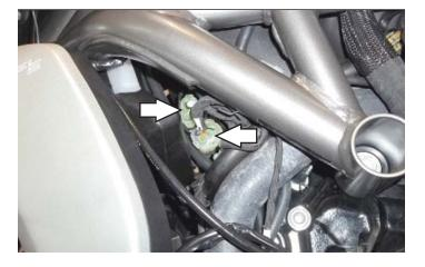
On the left side of the bike just behind the radiator, unplug the pair of stock 3-pin connectors labeled "INJ." Also unplug the pair of stock 6-pin connectors that are labeled "ETV".
