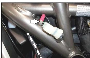
8 Unplug the stock Crank Position Sensor connectors.
