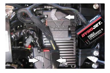
Plug the PC6 connectors in-line of the stock ECM and wiring harness.
