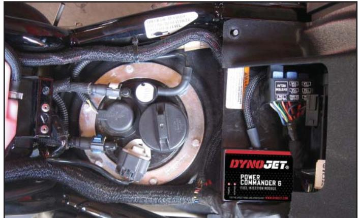
**USE THE FOLLOWING INSTRUCTIONS WHEN INSTALLING THE AUTOTUNE KIT P/N AT-100B.**
