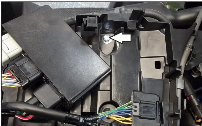
15 Pull the ECM rearward and unlatch it from its mounting bracket. Remove the bolt found beneath the ECM.
