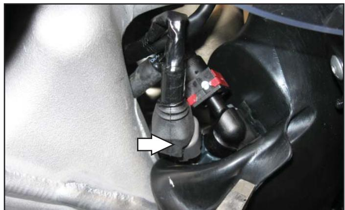
12 Plug the PC6 connectors with the YELLOW colored wires in-line of the stock wiring harness and the secondary fuel injector.
