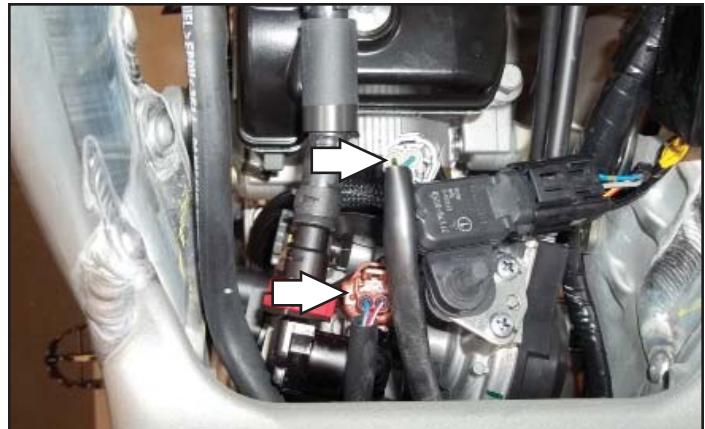
8 Plug the PC6 connectors with ORANGE colored wires in-line of the stock wiring harness and primary fuel injector. Plug the pair of PC6 3-pin connectors in-line of the stock throttle position sensor connectors.
