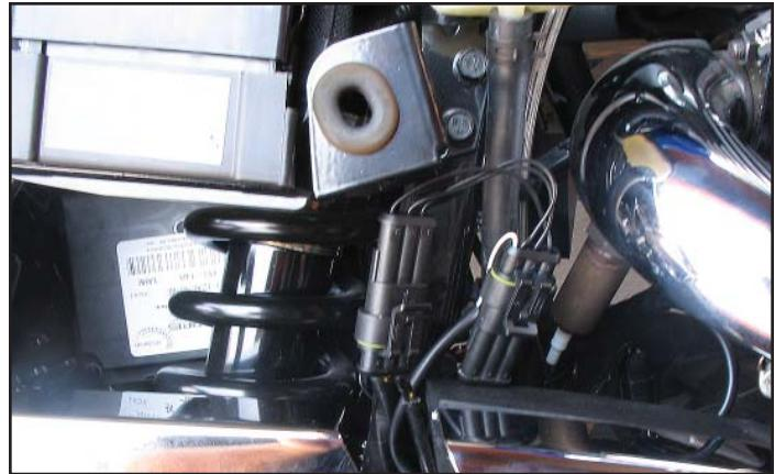
18 Attach the ground wire from the PC6 to the stock ground location which is on the inside of the left engine case.
