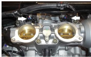
9 Plug the PC6 in-line of the stock wiring harness and injectors.
