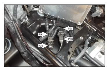
11 Plug the PC6 harness in-line of the stock CPS and wiring harness.
