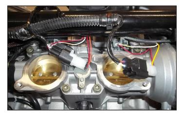
10 Locate the stock Crank Position Sensor connector and unplug it.
