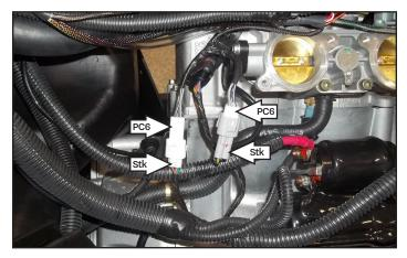
8 Unplug the stock wiring harness from both fuel injectors.
