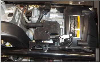
12 Locate and unplug the stock wiring harness from the Ignition Coil.
