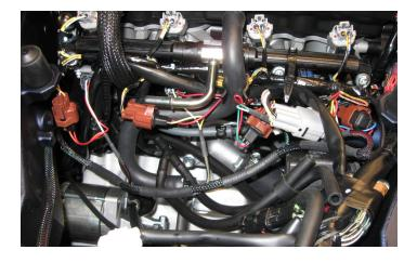
Plug the connectors from the PC6 in-line of the stock LOWER injectors and the stock wiring harness.
